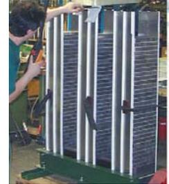
Partially assembled reactor with PolyGap™ core
