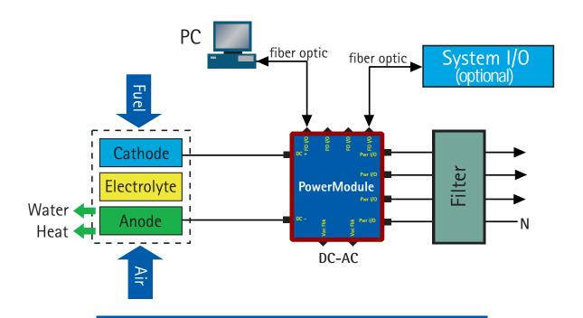
The PowerModule power converter is a scalable, state-of-the-art Power Electronic Building Block (PEBB) with a forward-looking architecture and self-supportive functionality for application ratings from 60 kW to several megawatts. It provides the following advantages:
